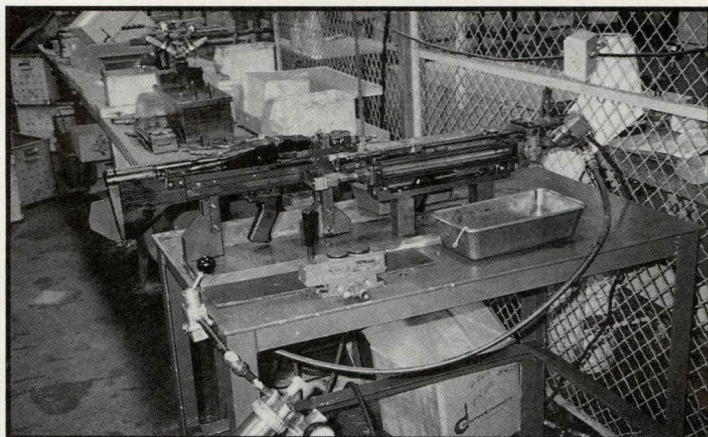
Pneumatic testing of the newly assembled machine gun breaks them in slow, and helps identify any fine tuning needed.
