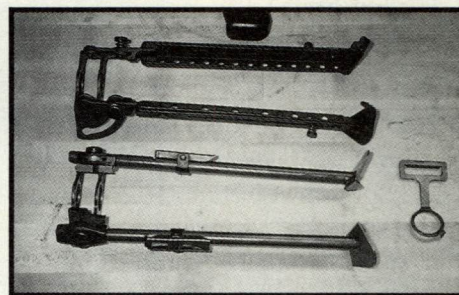
M60E3 flat bipod at the top, new M60E4 stronger, tubular design on the bottom.
