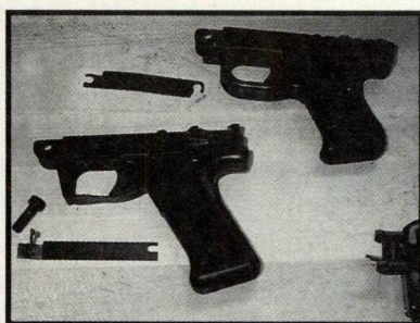
Top: M60 pistol grip/ trigger group with flat leaf spring that gets damaged. Bottom: M60E4 pistol grip/ trigger group with new flat spring, showing the capture pin. Note the slightly longer grip, and incline.
