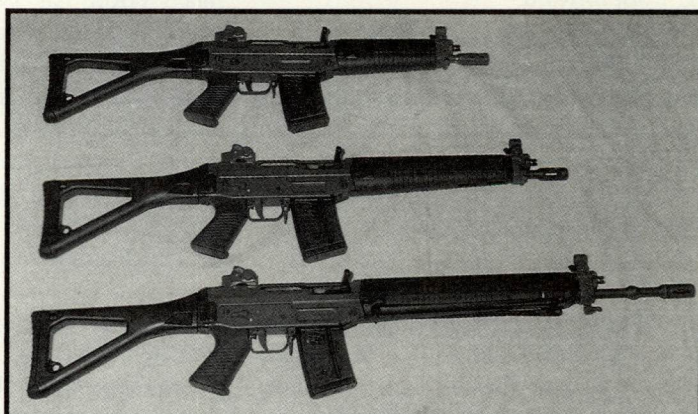
The picture shows the three SIG assault rifles 90. (Top to bottom): -short submachine gun version made by Brügger and Thomet; the dimensions are similar to the MP5, -short version (carbine made by SIG), -normal version with the bipod made by SIG for the Swiss Armed Forces.
