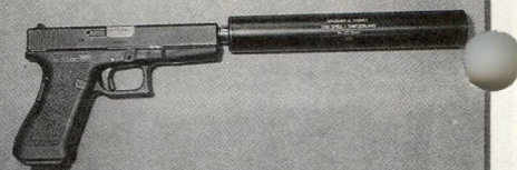
The famous Glock 17 pistol with an impulse silencer from Brügger & Thomet. It is the first silencer which works 100% reliable on this unique pistol.
