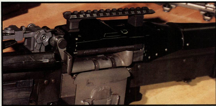
Note the body-bound rivet heads protruding from the receiver side, under the rear sight.
